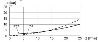
Q = f (n) Volume flow adjustment characteristics  $Q_N = 25 \text{ l/min}$
