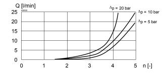
$\Delta p = f(Q)$  Flow-pressure loss characteristics Q = f(n) Volume flow adjustment characteristics  $2 \rightarrow 1$  through check valve throttle closed  $Q_N = 3.2$  l/min
